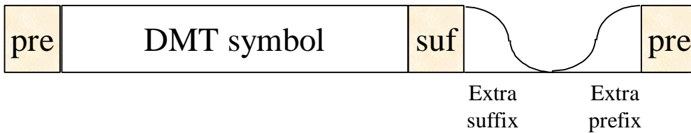
Figure 4a - Illustration of windowing in extra suffix/prefix samples - smooth connection of blocks without affecting necessary properties for digital duplexing.
