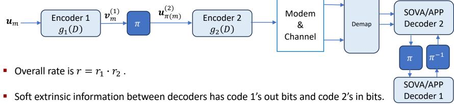
Initial soft intrinsic information is for code 2's channel/encoder output bits.
